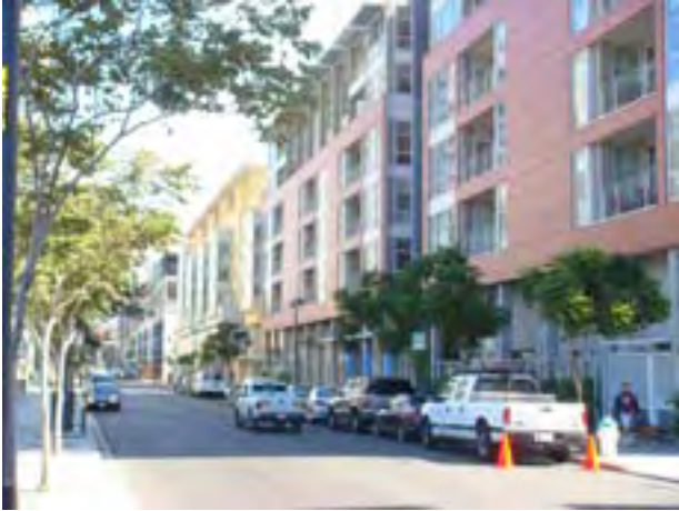
A significant portion of a street wall should be built to the setback line to create spatial definition along a street.
